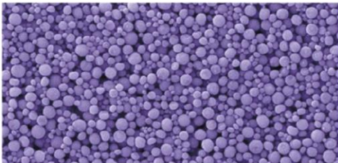
Figure 10: Scanning electron microscopy of nano-sized \text{TiO}_2 having particle size of 10–300 nm
